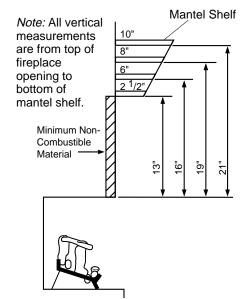
Figure 8 - Minimum Mantel Clearances for Built-In Installation
